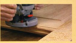
If you use a glass insert, rout away the stick profile on one side of the opening. Make new moulding with a similar profile to hold the glass in place.
