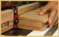
Before running the stick profile cuts, set up both infeed and outfeed stock supports. These supports are essential when running the long door stiles both from a safety and accuracy point of view. Also make sure your router table is completely stable with no risk of tipping. Now, run the stick profile cuts on the stiles. Remember that the profile is cut on one edge of the long stiles and and top and bottom rails; and on both edges of the shorter center stile and middle rail.
