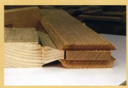
When running the panels, run the cross grain ends first and then the long grain sides. This will cut away any tear-out that may occur when exiting the cut on end grain. Also, keep good pressure both down and to the fence. Before making the final cut, use scrap to test cut the fit in the groove made by the sticking profile. It should be an easy slip-fit with no gaps showing. When running the final pass, consistent downward pressure is necessary to produce a consistently thick panel edge.
