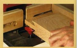
Repeat step 5 until you have produced a tenon with a total length 2½". Note in the photo above how the fences are almost fully closed to more fully support the work. When running the rails multiple times, keep good downward pressure on the work. You can make these multiple cuts easier by first removing some of the waste where the tenon is formed. Use a band saw to cut enough material so that the router bit is making more of a clean up and final cope cut instead of "hogging off" all the material.
