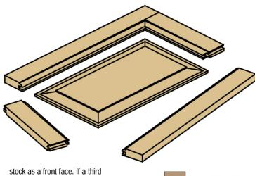
stock as a front face. If a third panel is required, mill one cut edge of the piece as instructed above, turn the piece over and run the other edge. Assemble the reverse cut pairs together for beautiful, strong joints that match up perfectly.
