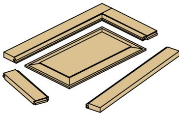
assures you will have the best side of your stock as a front face. If a third panel is required, mill one cut edge of the piece as instructed above, turn the piece over and run the other edge. Assemble the reverse cut pairs together for beautiful, strong joints that match up perfectly.
