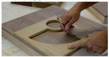
Lay out the bowl using the template. Center the template on the blank and mark the first partition. Remove the template and make marks exactly 1/2-in. from the edge of the first partition. This defines the wall thickness for each partition. It's important to be exact in order to achieve a uniform wall thickness for all the partitions. Use these marks to align the template for the two adjoining partitions. Make additional marks to position the template for the last partition.
