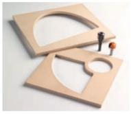
Glue up a bowl blank. Make an 18-in. x 18-in. blank to use with the round bowl template and a 15-in. x 23-in. blank for the oval template. Thick stock works best, but you can stack-laminate thinner boards to build the blank to the desired depth.
