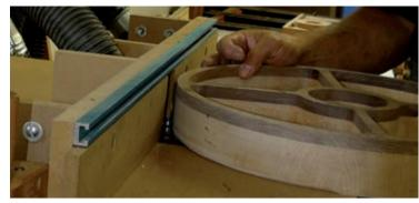
With the bowl sanded round and the band saw marks removed, head to the router table for some final shaping. Mount a 1/2-in. roundover bit in the router and round over the bottom edge of the bowl.
