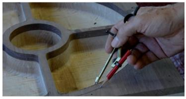
The next step is to lay out the outside wall of the bowl. Set a compass to mark a little over 1/2-in. to allow for sanding. Make sure the compass point extends about 1/4-in. or so past the pencil point.
