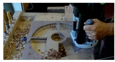
Secure the blank to your bench. With the plunge mechanism set at the top of its travel, place the router over an open area on the template. Make sure the cutter is not contacting the wood and turn on the router. Gently slide the router to the template edge and begin your cut. Continue the cut around the opening. Then, lower the bit 3/8-in. and make another pass. Eventually the bearing on the bit will
