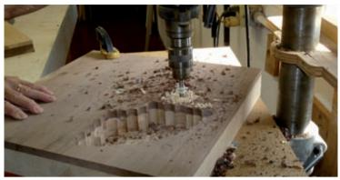
Use a Forstner bit in a drill press to remove most of the wood. Forstner bits do the best job because they can make overlapping cuts and leave a flat bottom.
