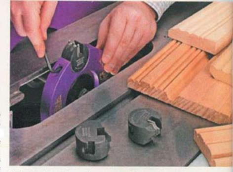
▲ The Magic Molder makes cutting molding on the table saw easy. You can even change cutters while it's still mounted on the saw.
